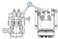
Depending on the model of pump, the check valves are located on either the side or top of the manifold.
