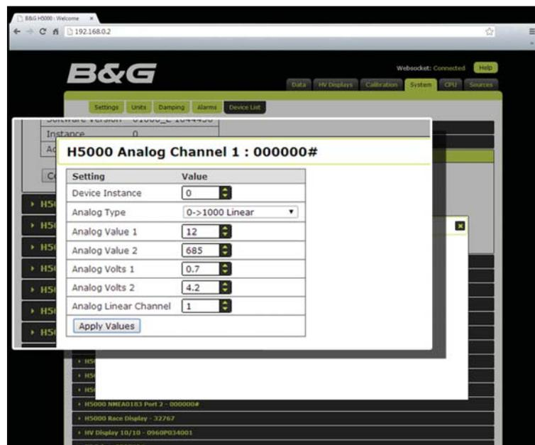
→ **Note:** Analog linear channel is the channel on the display where the data is sent to. There are user channels available.
