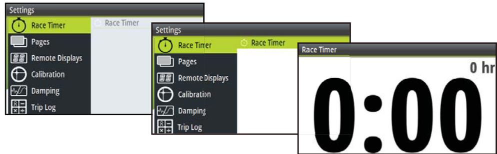
→ **Note:** The timer set value is in Hours : Minutes (hh:mm), the timer counter will show Minutes : Seconds (mm:ss) with the hours shown in the top right hand corner of the display.
