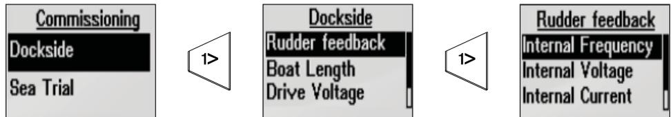
→ **Note:** Select External for network sources or Internal frequency for RF300 sensors.
