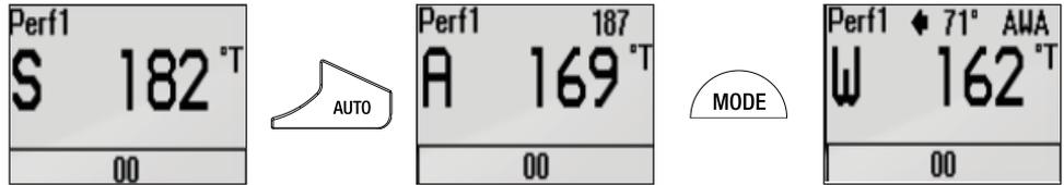
To access other autopilot modes press and hold the **MODE** key for 2 seconds. Highlight the required mode and press the **1° RIGHT** key to confirm.
