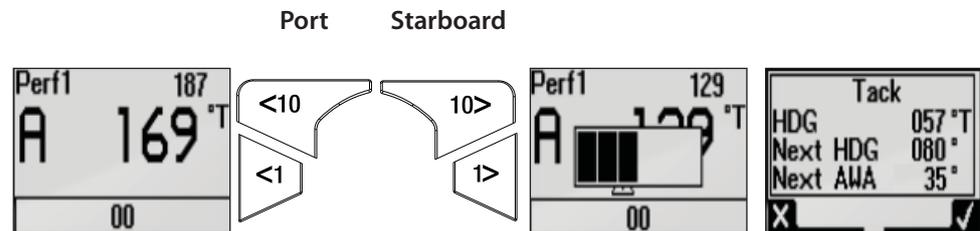
The rate of turn during the tack/gybe is set by the Tack time parameter in the Setup/Sailing menu. The change in heading is controlled by the tack angle parameter in the Setup/Sailing menu.
