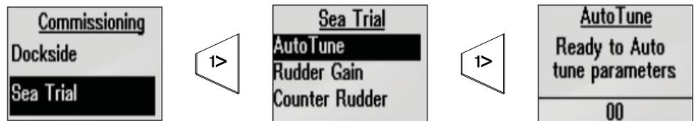
The automatic tuning process is also verifying/adjusting the Rudder zero alignment made in Dockside setup.
