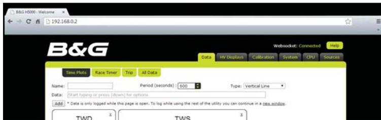
→ **Note:** It will say “Websocket: Connected” in the top right-hand corner of the screen next to the help tab. If it says “Websocket: Not Connected” then check the H5000 CPU and router power and connections.
