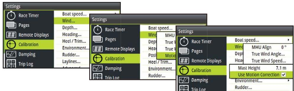
➔ **Note:** A 3D Motion sensor and mast height value is required in conjunction with a CPU running Hercules level software or greater to use this feature.
