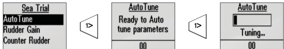
After the Autotune has been completed the rudder must be controlled manually, as the autopilot has returned to Standby mode. The Automatic tuning function will take control of the boat and perform a number of S-turns.
