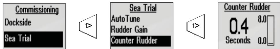
The best way of checking the value of the Counter Rudder setting is when making turns. The figures illustrate the effects of various Counter Rudder settings.
