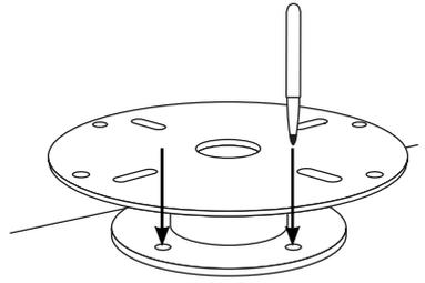
**2** Using a 5/16" (8mm) drill bit, drill the four base bolt holes and center cable hole.
