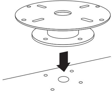
**6** Using your own bolts and the provided nylon shoulder washers secure the mount. Apply marine adhesive sealant to the threads.
