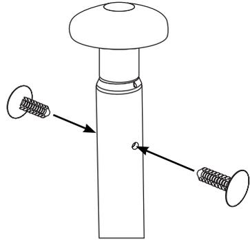
**4** When securing make sure that LTBU or LTBUSS is facing forward. To check this line up the notch on the LTBU or LTBUSS with the hole on the back of the light bar as shown.
