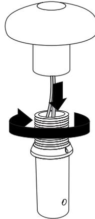
**2** Apply marine adhesive sealant to the LTBU or LTBUSS as shown. Be sure to apply around the push pin hole as well.
