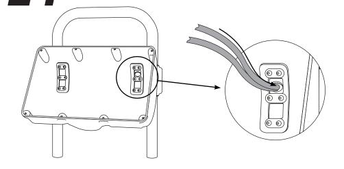
Install the rubber gasket and lid assembly on to housing. Note that the rubber gasket may already be installed onto the front face plate.
