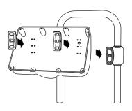
Secure the backing plate with the M4 x 0.7 x20mm bolts.
