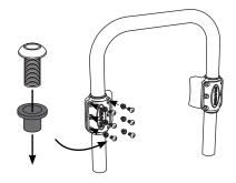
Place the white plastic backing plate in the SPOD housing as shown.
