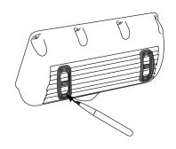
Use a 6mm drill bit to drill out the holes you just marked.
