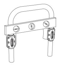
Secure the clamp assembly with the twelve black nylon shoulder washers and twelve M6x1x15mm bolts.
