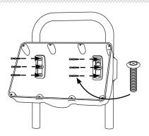
Place the instrument template onto the lid of the SPOD.
