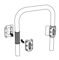
Secure the clamp assembly with the twelve black nylon shoulder washers and twelve M6x1x15mm bolts.
