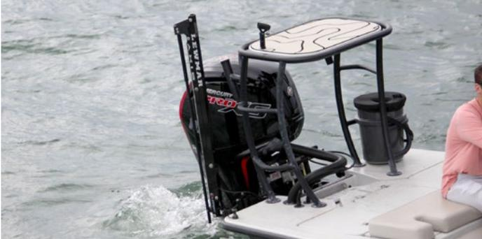
With no hydraulic pump and hoses to worry about the shallow water anchor can be installed quickly and takes up less space.
