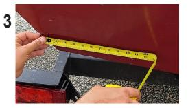
Find the proper location for the *HydroPlane*. Measure 3-5" in from the outside edge of the boat or position just inside the first chine.
