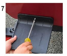
Using the 1/4 x 1 sheet metal screw, Slide the screw through the black washer and then install the plate using a Phillips head screw driver. DO NOT use a drill gun as vou risk breaking the screw head. IMPORTANT NOTE: Make sure you tighten down the screws all the way, as tight as you can get them by hand.
