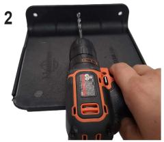
Using a 7/32 drill bit, drill out the location markers. **NOTE:** Run the drill bit in and out 2-3 times to smooth out the hole.
