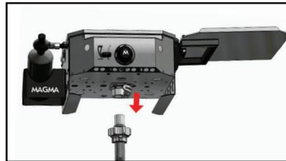
**5** – Place the Firebox or Grill onto the mounting arm.
