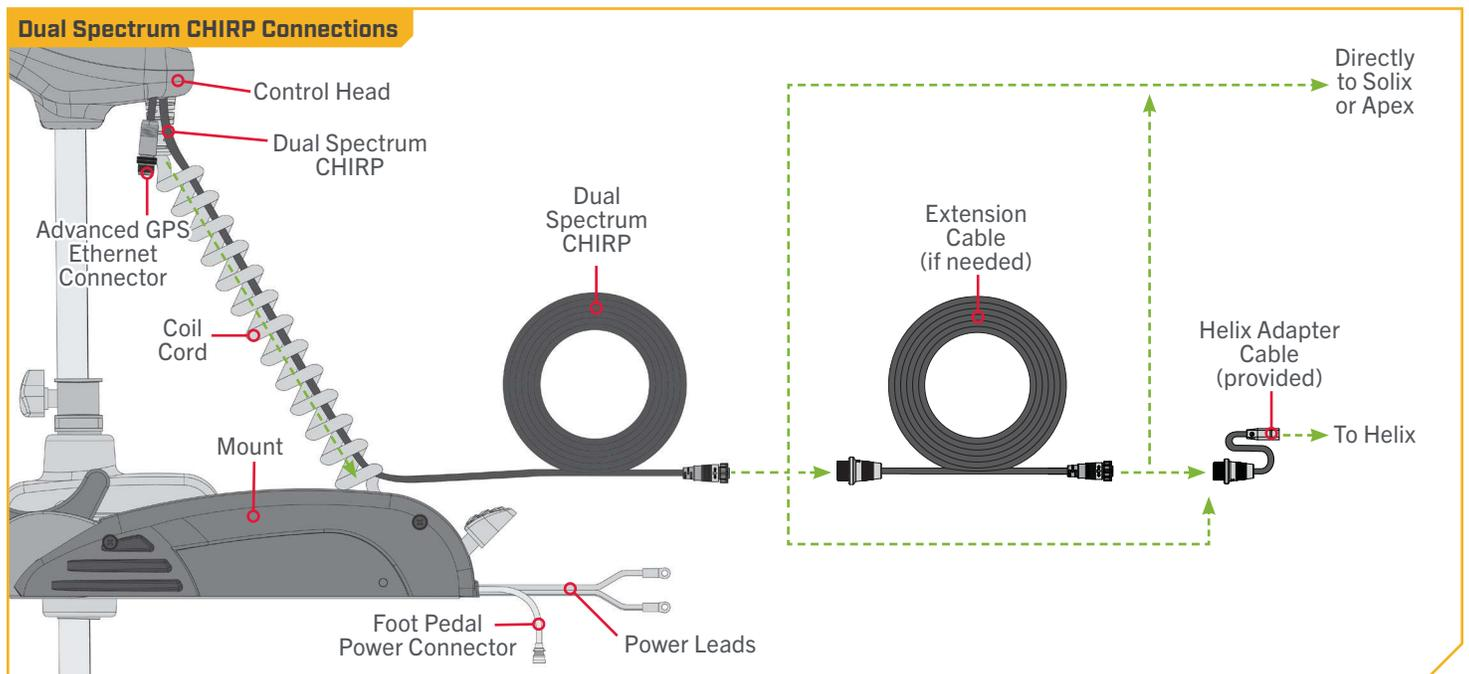
All Dual Spectrum CHIRP Terrova motors are equipped with an internal bonding wire. Incorrect rigging will cause sonar interference and can damage your trolling motor, electronics, and other boat accessories. To minimize trolling motor interference, ensure that the fish finder and trolling motor are powered by separate batteries. Please refer to the "Battery & Wiring Installation" and "Motor Wiring Diagram" sections of this manual for correct rigging instructions.
