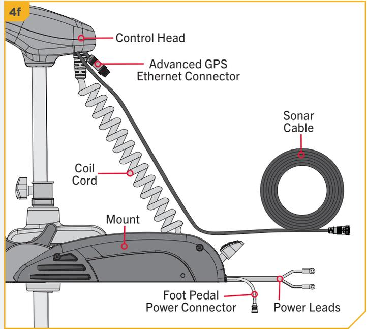
**NOTICE: CRITICAL CABLE ROUTING.** On motors with a shaft 60" or more, accessory cables must exit the Coil Cord leaving three or more open coils between where the cables exit and the motor base, as assembled by the factory. Routing the cables in any other manner will not allow the motor to stow properly. Please see the “Securing Accessory Cables” section of this document for details.
