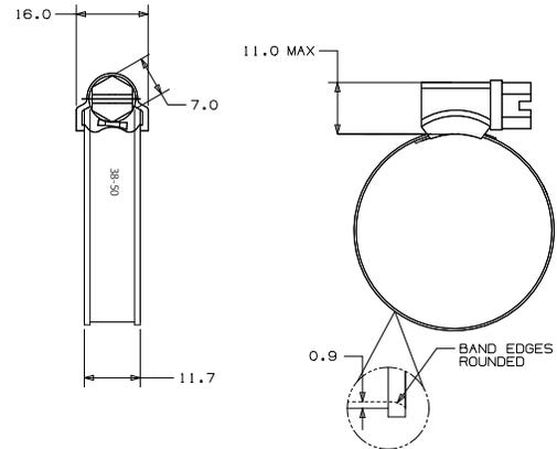
Premium Marine Grade, all AISI 316 (high tensile strength) Stainless Steel “HD NON-PERF” Worm Gear Hose Clamp. The 11.7 mm (0.46”) wide band is Non-Perforated and Smooth on the inside with Rolled Edges. This eliminates hose damage with increased clamping force. The High Strength, Compact, One Piece 16mm (0.63”) wide Housing provides one of the highest clamping force ratings of any worm gear style clamp. Screw Head is 7mm.
