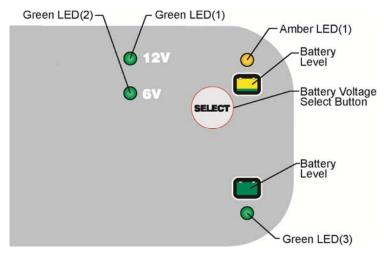
When AC power is first applied to the charger all of the LEDs will illuminate for two to three seconds before starting the charge sequence listed below.
