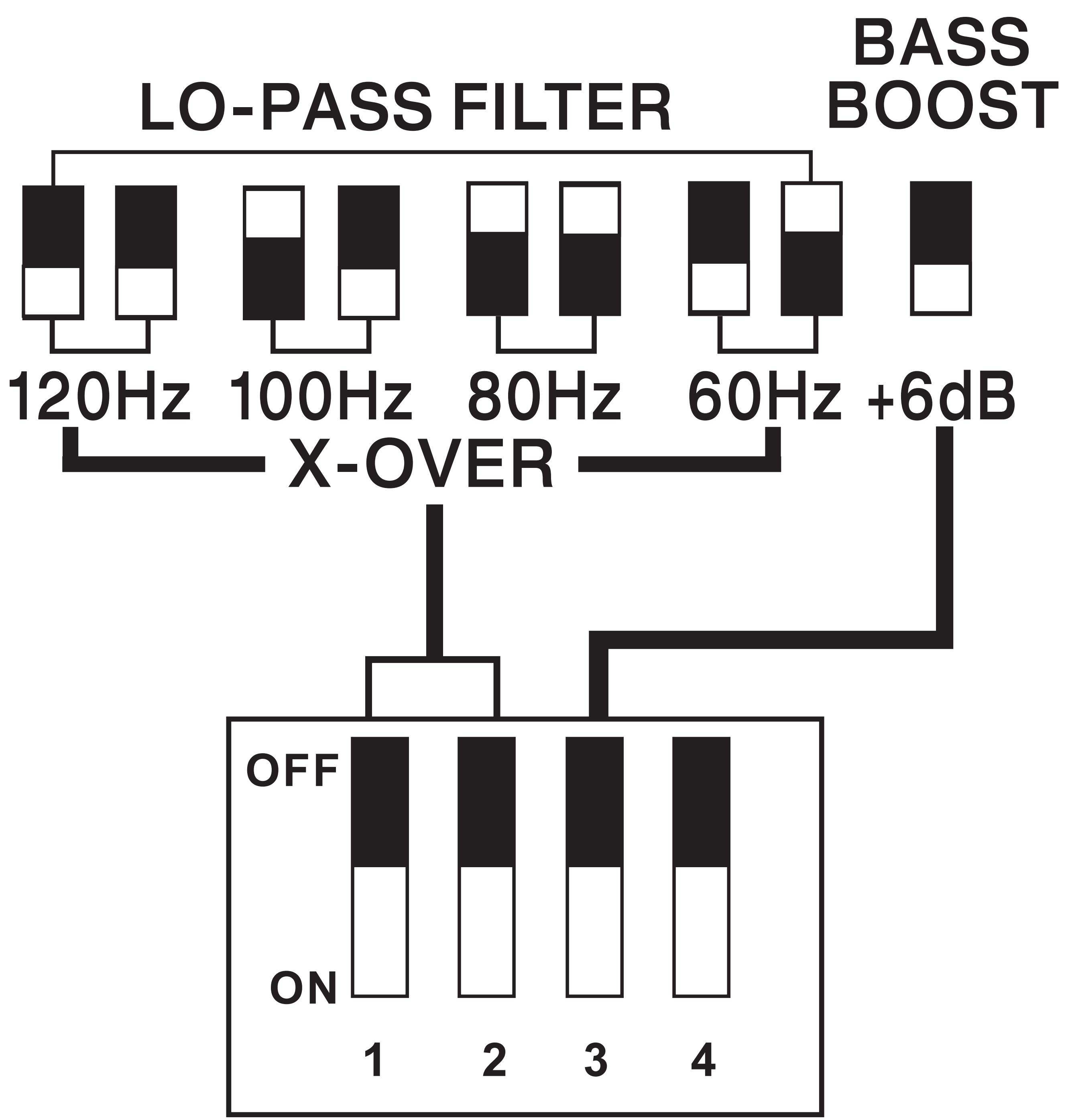
**KICK EQ Bass Boost:** The bass boost is designed to give you increased output, +6dB, at 40Hz. If you turn it on, you must readjust the input gain control to avoid clipping the amplifier.
