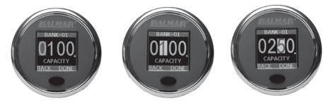
Once you select a chemistry, you must specify the capacity of the battery bank. This is the total design capacity of the entire bank, regardless of the battery's condition, or previously measured capacity. Typically the capacity is expressed as the 20-hour discharge rate. This may be written as something like "105Ah/20h" on the battery or battery documentation. If you cannot find
