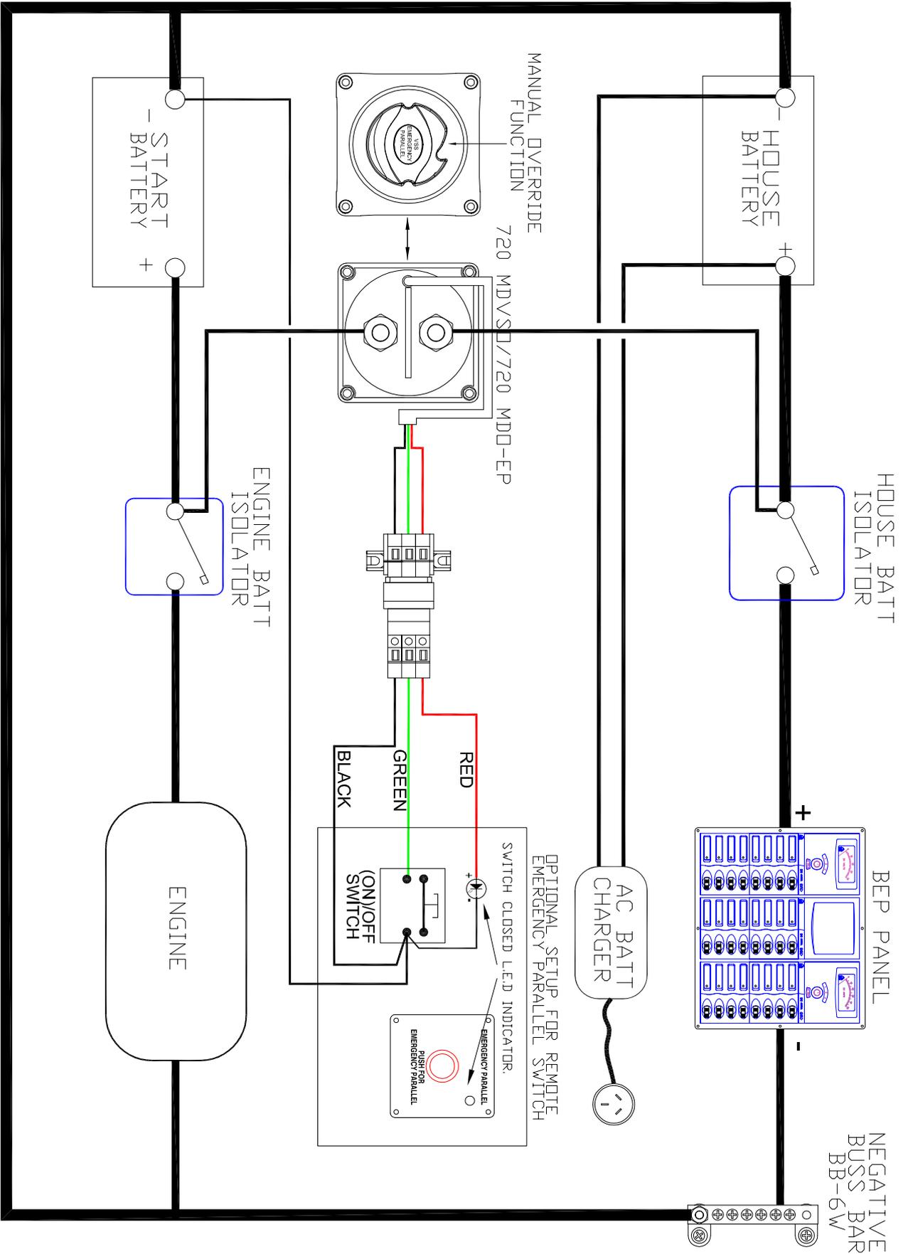
IT IS IMPERATIVE THAT THE NEGATIVE (BLACK) FOR THE MDO-EP/MDVSO IS TAKEN FROM THE SAME BATTERY THAT IT IS ISOLATING. FAILURE TO DO THIS WILL CAUSE THE UNIT TO WORK ERRATICALLY. ONLY ONE NEGATIVE MUST BE SUPPLIED TO EACH UNIT FOR CORRECT OPERATION.
