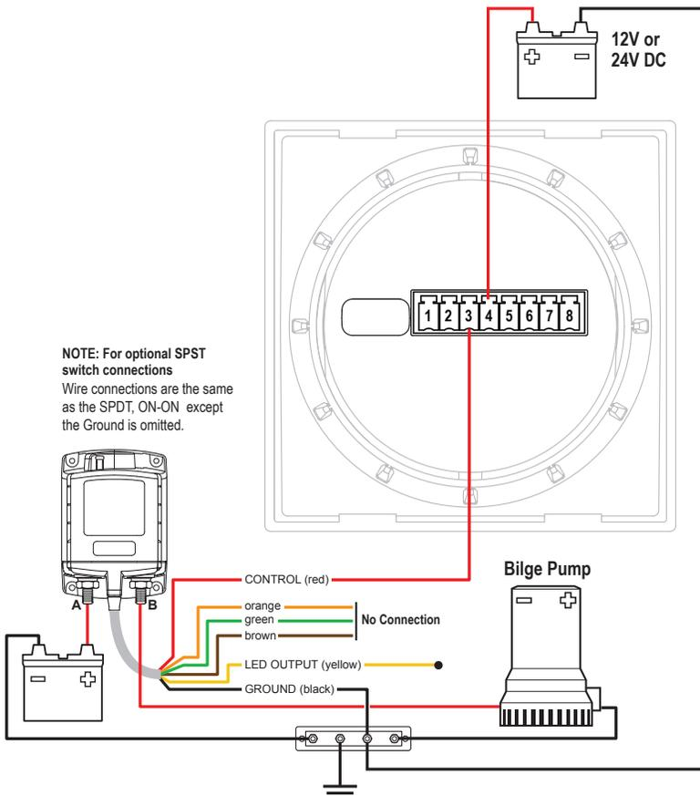
**NOTE:** 9012, 7700, 7701, 7702, & 7703 Remote Battery Switches are not compatible with the internal relay.
