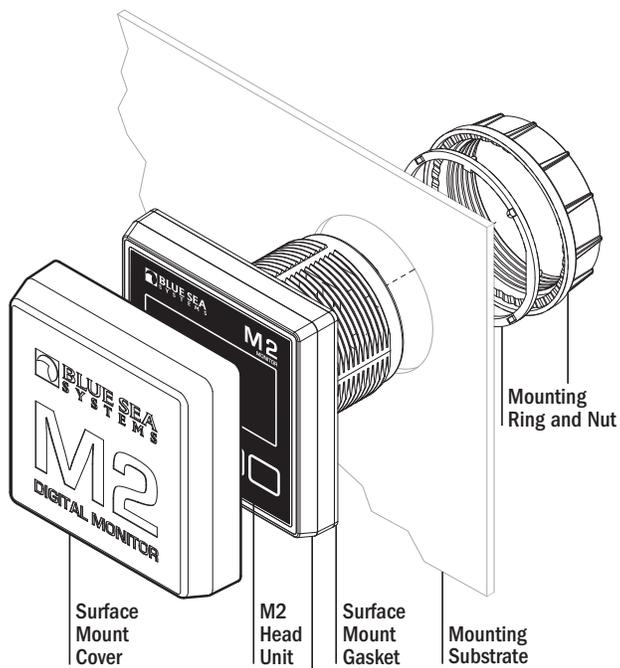
**NOTE:** During installation use cover to align the bezel and gasket
