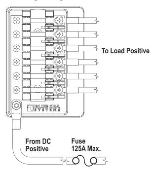
Application Note: This device is intended for branch circuit protection. Suitable main circuit protection of not more than 125A rating should be provided ahead of this device with an interrupt current rating consistent with the battery capacity. Consult ABYC E-11 Table V See "Circuit Protection" at www.bluesea.com.
