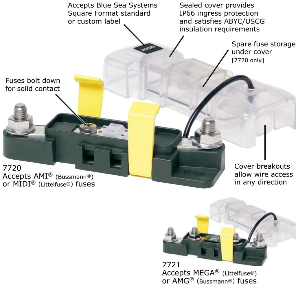
The Safety Fuse Blocks fulfill a need for in-line main or branch circuit protection for 30A – 200A circuits (AMI®/MIDI®) and 100A – 300A circuits (MEGA®/AMG®).
