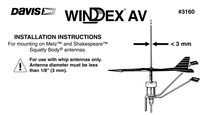
Adjust reference tabs. Bend the tab support wire to the proper angle using the reference tab template included in the packaging and reproduced here at half size. Tabs should be adjusted before ascending the mast.
