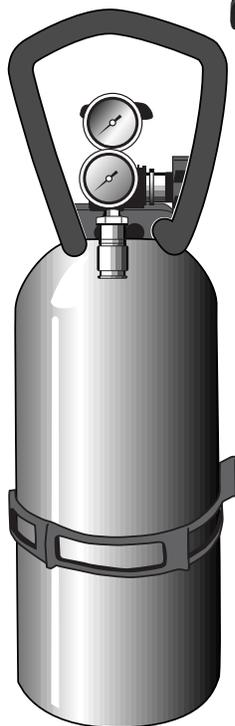
If you plan on holding a large cylinder with the base unsupported, it is advisable to use a piece of angle iron, wood block or shelf bracket at the bottom of the cylinder. This will prevent slippage (especially on a vehicle) and will also make it easier to lock the clamp in place.
