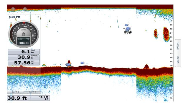
We recommend using a screen advance of 1/1, TX rate setting to 20 and if you need to use Interference Rejection, use a Medium setting. You can also try using a black background for better target contrast. Good fishing.
