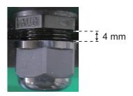
8. Position the cable so its vinyl sheath lies in the cable clamp. Use the supplied cable clamping plate to secure the cable.
