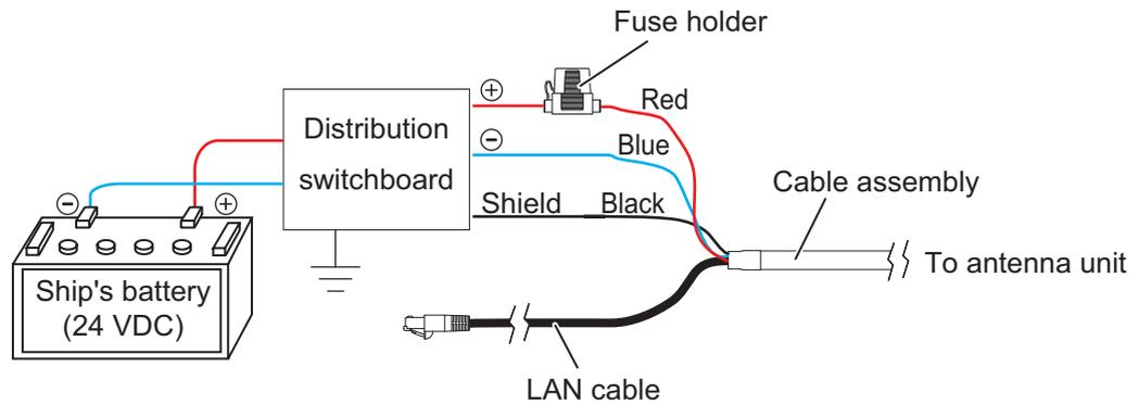
**Note 1:** The antenna unit has no power switch. Connect the antenna unit to a distribution switchboard with a switch for power control.
