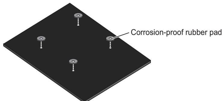
3. Apply silicone rubber to the thread of the stud bolts (M12×70, 4 pcs).
