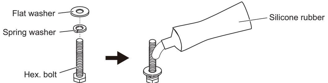
6. Fasten the radiator to the radiator bracket, using four bolt assemblies prepared at step 5.
