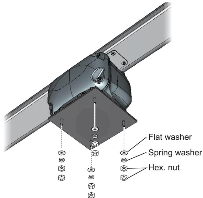
8. Apply silicone rubber to the flat washers, spring washers, and hex. nuts.
