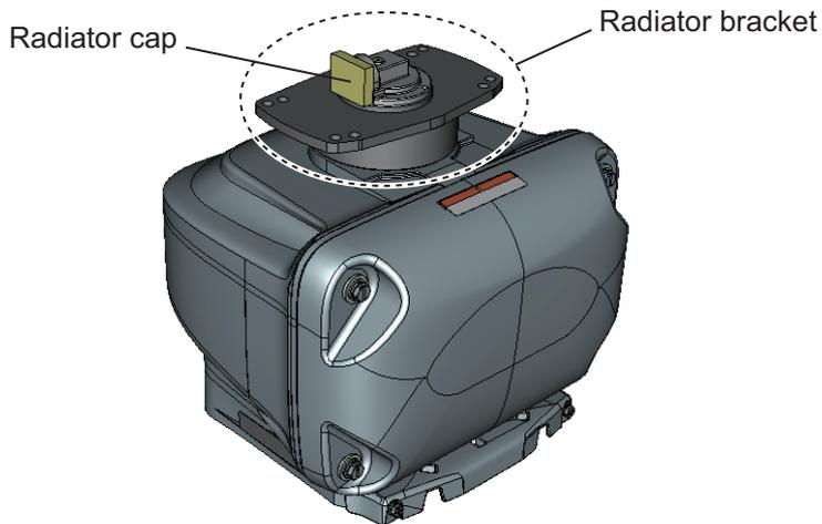
2. Apply silicone rubber to the surface of the radiator bracket as shown in the figure below.
