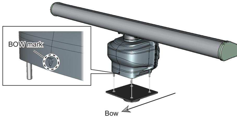
7. Secure the antenna unit, using the supplied flat washers (M12, 4 pcs), spring washers (M12, 4 pcs), and hex. nuts (M12, 8 pcs).
