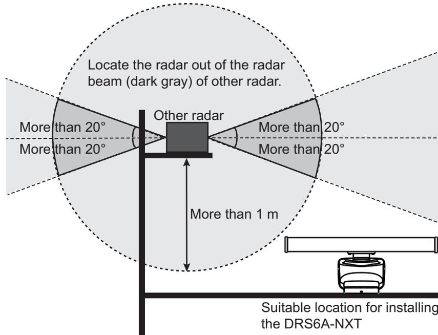
**Installation with the radiotelephone equipment**
