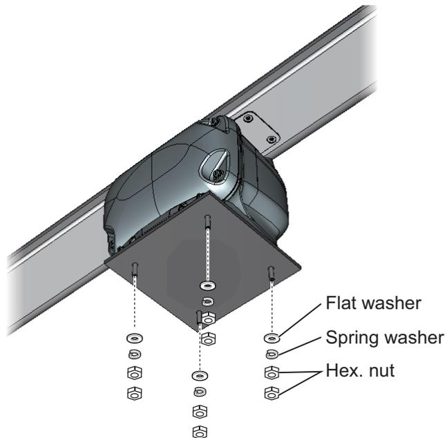
8. Apply marine sealant to the flat washers, spring washers, and hex. nuts.
