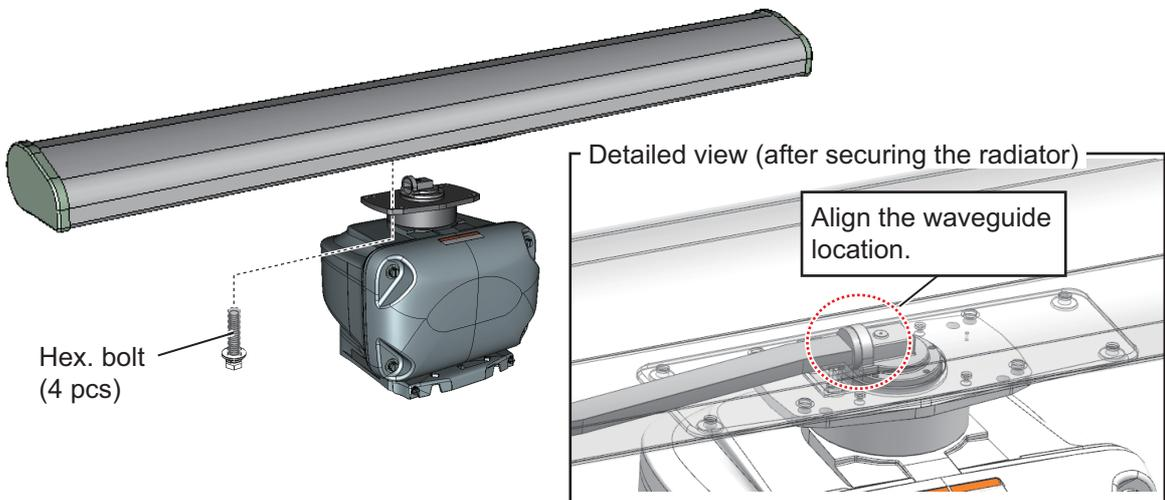
7. Apply marine sealant to the holes and bolts at the locations indicated with arrows in the figure below. Also apply marine sealant to the junction between the radiator and the radiator bracket.
