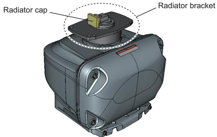
2. Apply marine sealant to the surface of the radiator bracket as shown in the figure below.
