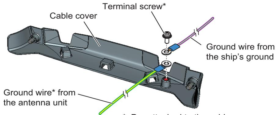
5. Apply marine sealant to the ground terminal after fastening the terminal screw.
