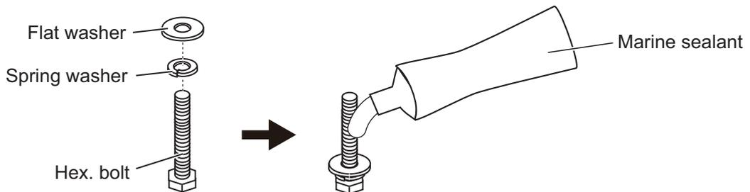
6. Fasten the radiator to the radiator bracket, using the four bolt assemblies prepared at step 5.
