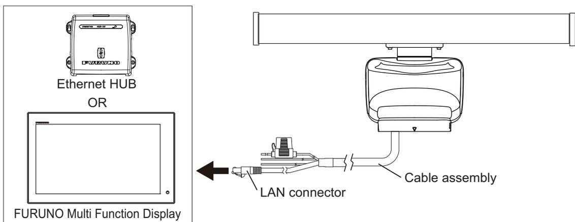
**Note 2:** When LAN cable extension is needed, use the optional LAN cable (MOD-Z072) and joint box (TL-CAT-012). After connection is completed, wrap the connector with vinyl tape to waterproof the LAN connector.
