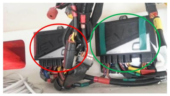
2. Locate the "MULTI LINK" bus cable or find an Open Port on an EVC Bus connector to make the VP IPS Gateway Connection. The bus cable connections and hub (if installed) will be located close to the EVC unit.
