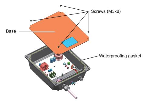
3. Confirm that the LED on the board is OFF, and then replace the fuse.
