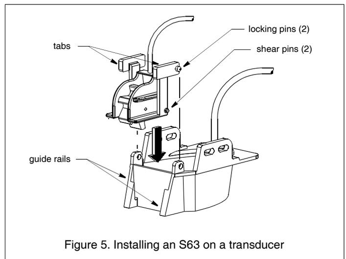
Figure 5. Installing an S63 on a transducer
