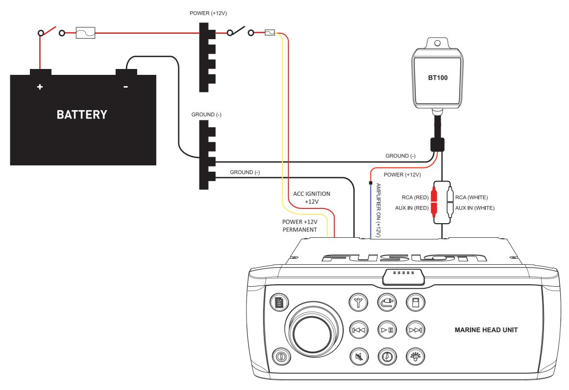
**NOTE:** MS-BT100 is compatible with any stereo with an AUX IN In instances where the AMPLIFIER ON cable is not provided, simply wire the POWER +12V cable of the MS-BT100 to the POWER +12V of the connecting stereo.
