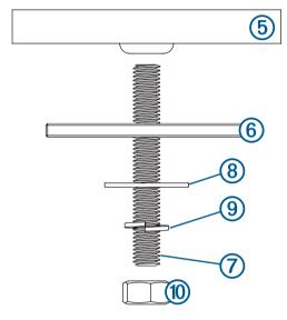
**9** Using a torque wrench, tighten the nuts from 13.7 to 18.6 Nm (10 to 14 lbf-in.) of force.
