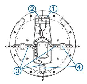
3 Press the cables into any of the guide grooves ③ on the bottom of the case, and secure them using a cable holddown plate ④. The cables should be bent or twisted as little as possible.
