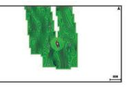
A green circle indicates good depth and GPS position, and a speed under 16 km/h (10 mph). A yellow circle indicates good depth and GPS position, and a speed between 16 and 32 km/h (10 and 20 mph). A red circle indicates poor depth or GPS position, and a speed above 32 km/h (20 mph).
