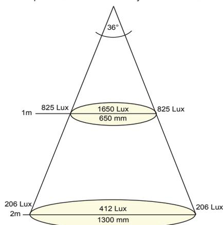
Wide Spread Luminous Intensity - Distance / Lux
