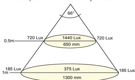
Spread lamps offer higher light intensity while the Wide Spread lens is better for applications with confined spaces or that require extra wide spread of light.
