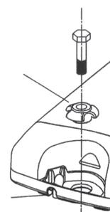
Completely sealed unit with robust bush mount.
