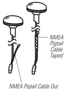
4. Route the Sensor cable through the stem and through the planned cable route. To use extension cables, see the details in **Section 1: Choose the Mounting Location**.
