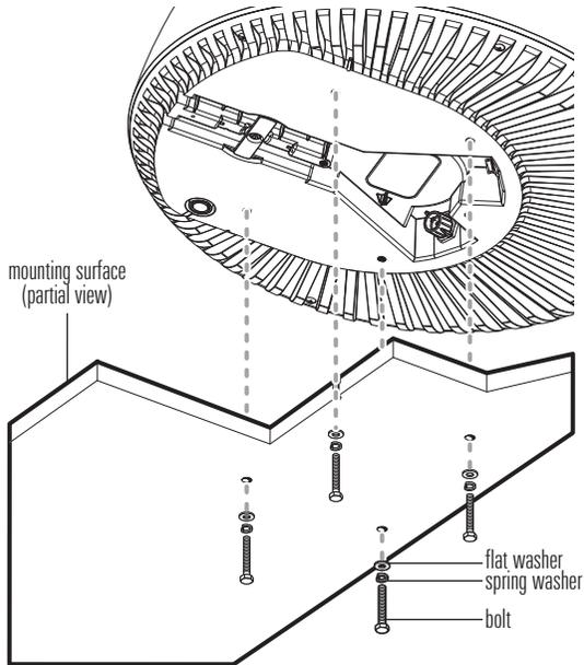
6. Hand-tighten the bolts to a torque of 11 ft-lbf (15 Nm).
