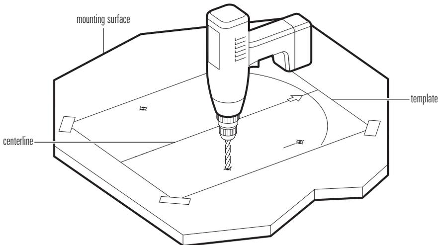
8. **Test the hardware:** Check that each bolt (with spring washer and flat washer) protrudes through the mounting surface at least 5/8" (16 mm) but less than 7/8" (22 mm).
