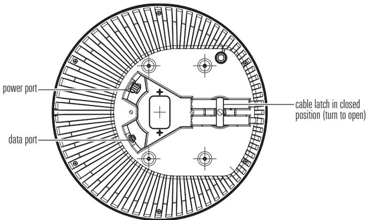
5. Connect the power cable connector to the power port on the Radar scanner, making sure that the notch lines up with the guide in the port.
