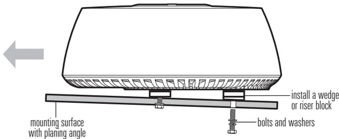
3. Install one spring washer and one flat washer on each bolt as indicated in the illustration *Mounting the Scanner Unit*.
