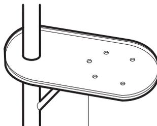
Do not mount on a surface with an edge that might trap water.
