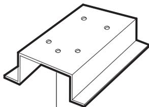
mounting surface is clear and doesn't trap water
